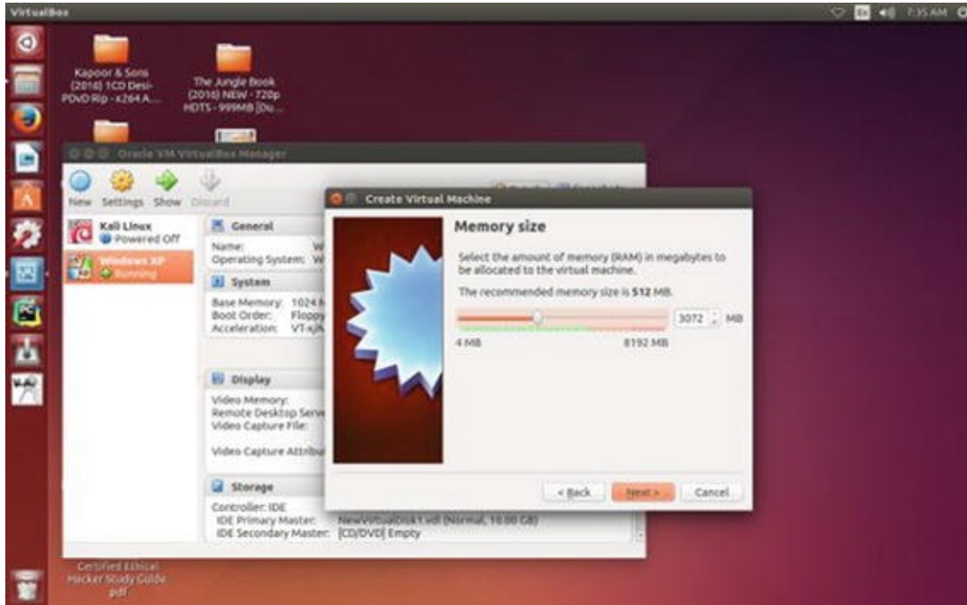
Figure 4-2. Installation process of Kali Linux on Virtual Box asks for memory size
