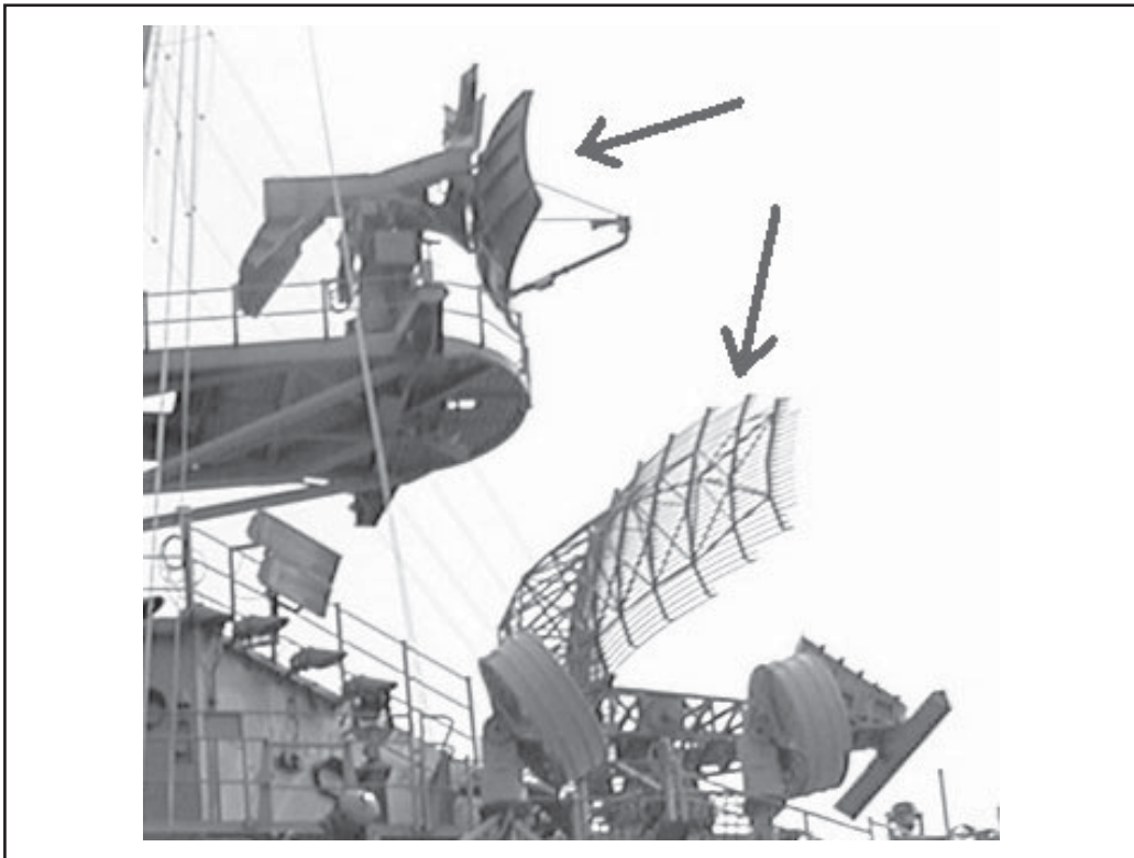
Figure 8-5 Parabolic grid antennas on U.S.S. Enterprise CVN-65 (photo courtesy of Julian “HammerJammer” Ho)
